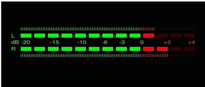
Fig. 3.3: VU- metro de leds
